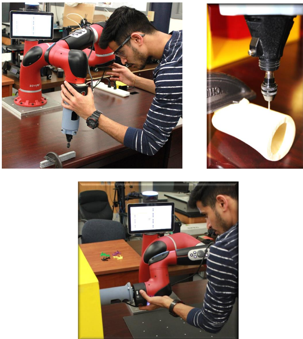
Fig. 1. 2 Human robot collaboration and drilling in Complex orientations
