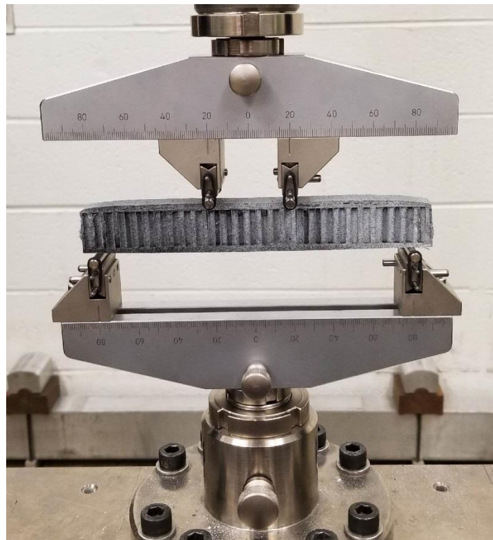
Fig. 4. 3 Test setup (four-point bend test)
